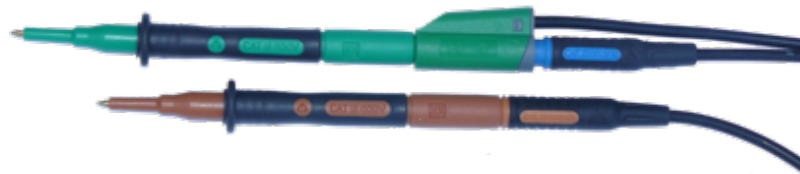
Fig 3. Prods in 2 wire testing configuration
