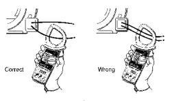
d. Press the trigger to open the transformer jaws and clamp them onto the conductor under test and take the reading on the display
