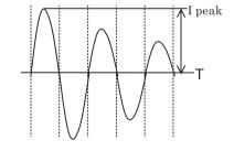
(4) Press the PEAK Key at least 2 sec to reset the indication or release PEAK Function. Buzzer sounds twice, and the Function is released.
