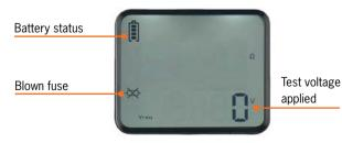
The LCD is shown indicating a blown fuse
