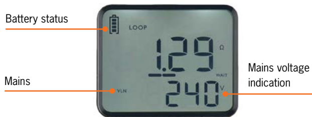
LCD display shown in the no trip loop function.
