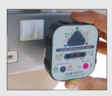
Flashing red LED with warbling means the earth path is over  $93\Omega$ . This may not be dangerous but the value should be checked using an earth loop tester with a read out to check the value meets the wiring regulations.
