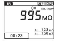
10 This instrument has an auto-discharge function. With the test leads connected to the circuit under test, release the Test button to discharge capacitance in the circuit after test.
