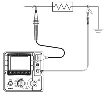
Put the tip of the Line Probe (red) to the circuit under test. Then press the Test Button. The buzzer sounds intermittently during a measurement.
