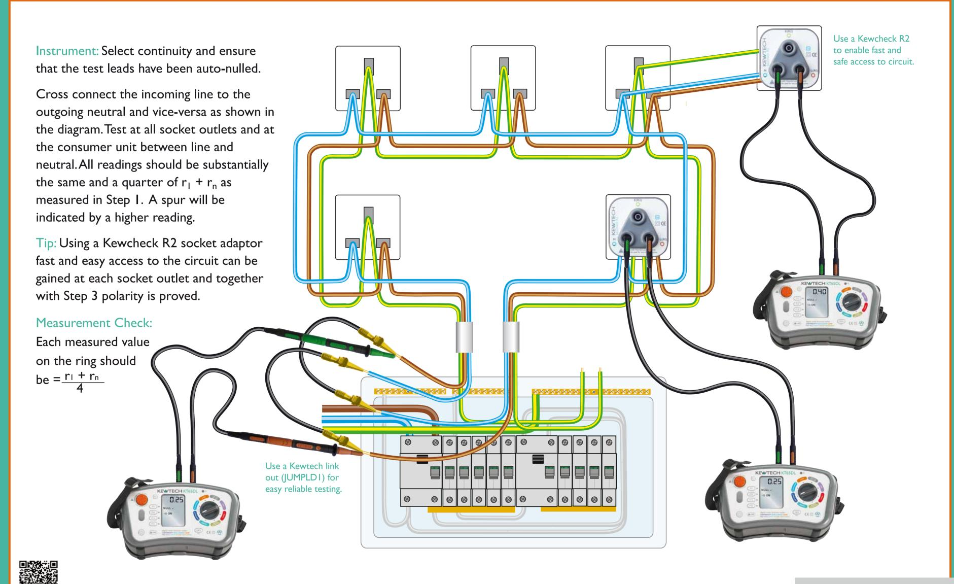
Kewtech 'Clear Thinking' diagrams are schematics to aid the understanding of electrical testing. Ensure proper safety procedures are taken before any testing.
