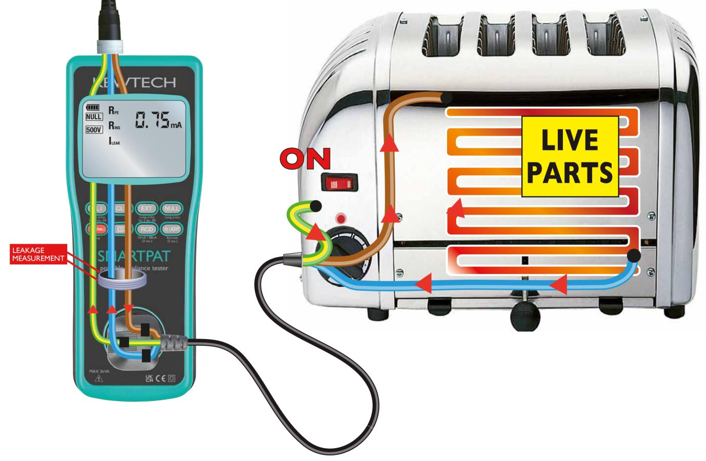
Kewtech 'Clear Thinking' diagrams are schematics to aid the understanding of electrical testing. Ensure proper safety procedures are taken before any testing.
