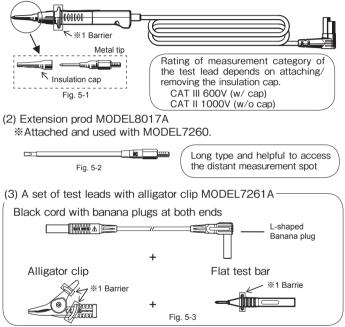
%1 Barrier is a part providing protection against electrical shock and ensuring the minimum required air and creepage distances.
