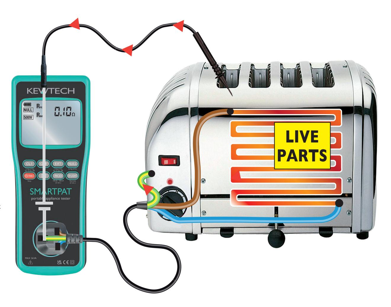
Kewtech 'Clear Thinking' diagrams are schematics to aid the understanding of electrical testing. Ensure proper safety procedures are taken before testing.
