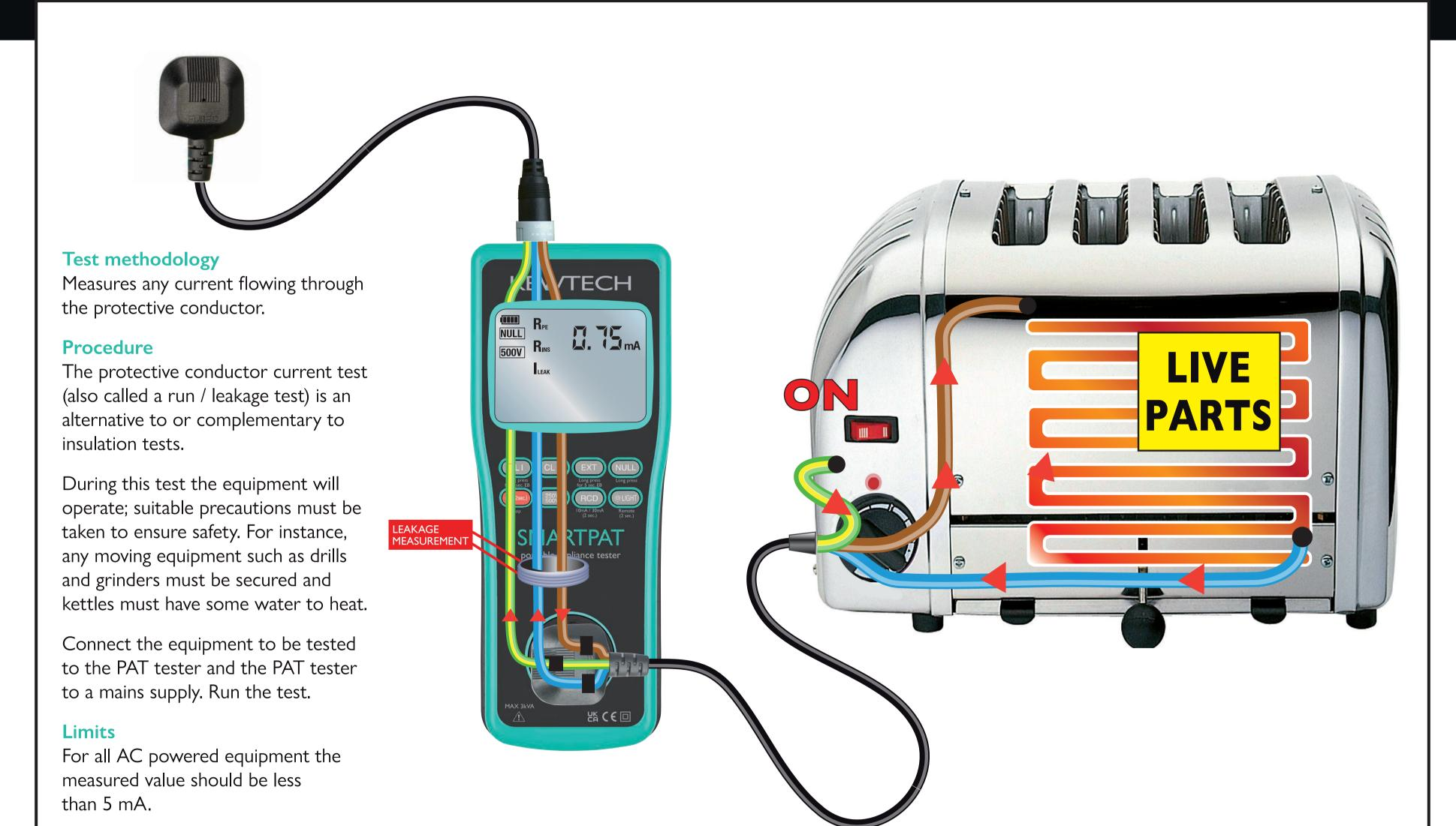
Kewtech 'Clear Thinking' diagrams are schematics to aid the understanding of electrical testing. Ensure proper safety procedures are taken before testing.
