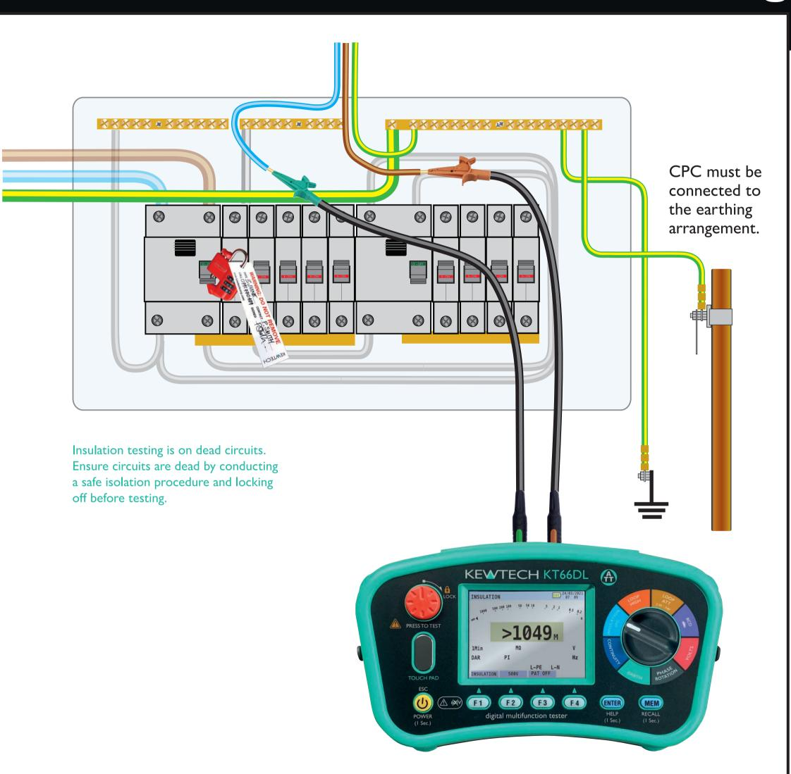
Kewtech 'Clear Thinking' diagrams are schematics to aid the understanding of electrical testing. Ensure proper safety procedures are taken before testing.
