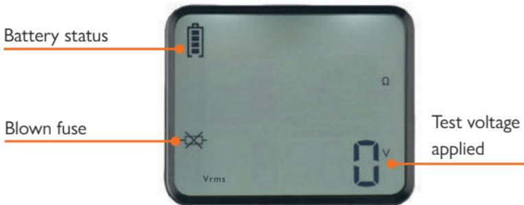
The LCD is shown indicating a blown fuse
