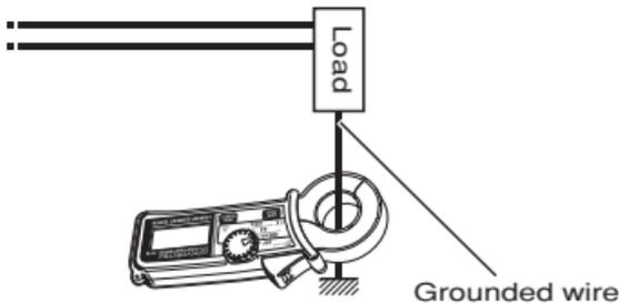
Fig.2 Measuring earth leakage current
