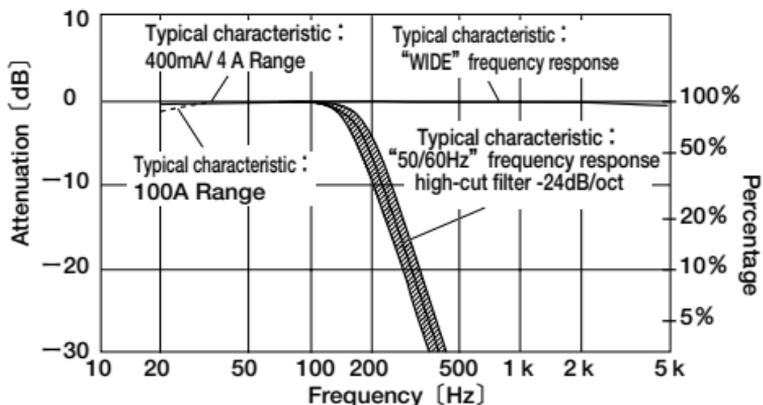
Fig.3 Model 2434 Frequency Characteristic
