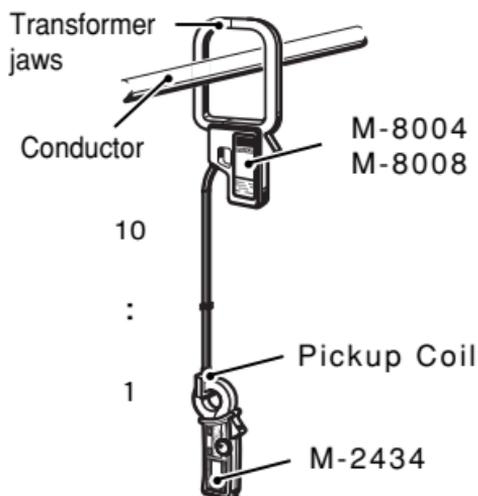
Note: Model 8004 and Model 8008 cannot be used for leakage current measurement. For detailed specifications, refer to the instruction manual for Model 8004 or Model 8008.
